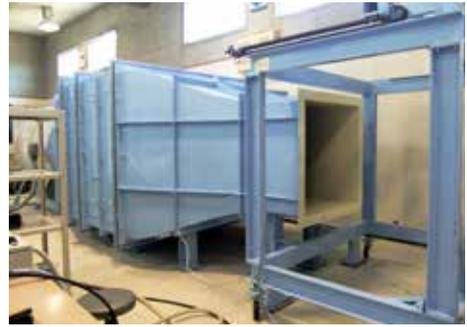
The facility is shared by all the departments and mainly used for fluid dynamics experiments. Also it is used for graduation research of Department of Mechanical Engineering and Advanced Engineering course.
